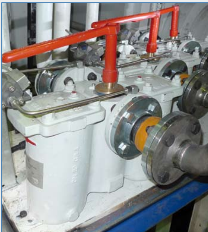
Fig. 4 Duplex Filter in cast iron design
